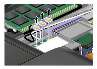
**Note:** Depending on the model, if your computer has the Multiple Input Multiple Output (MIMO) feature, the wireless LAN card has three connectors as shown in the above figure. If your computer does not have the MIMO feature, the wireless LAN card might have only two connectors.
